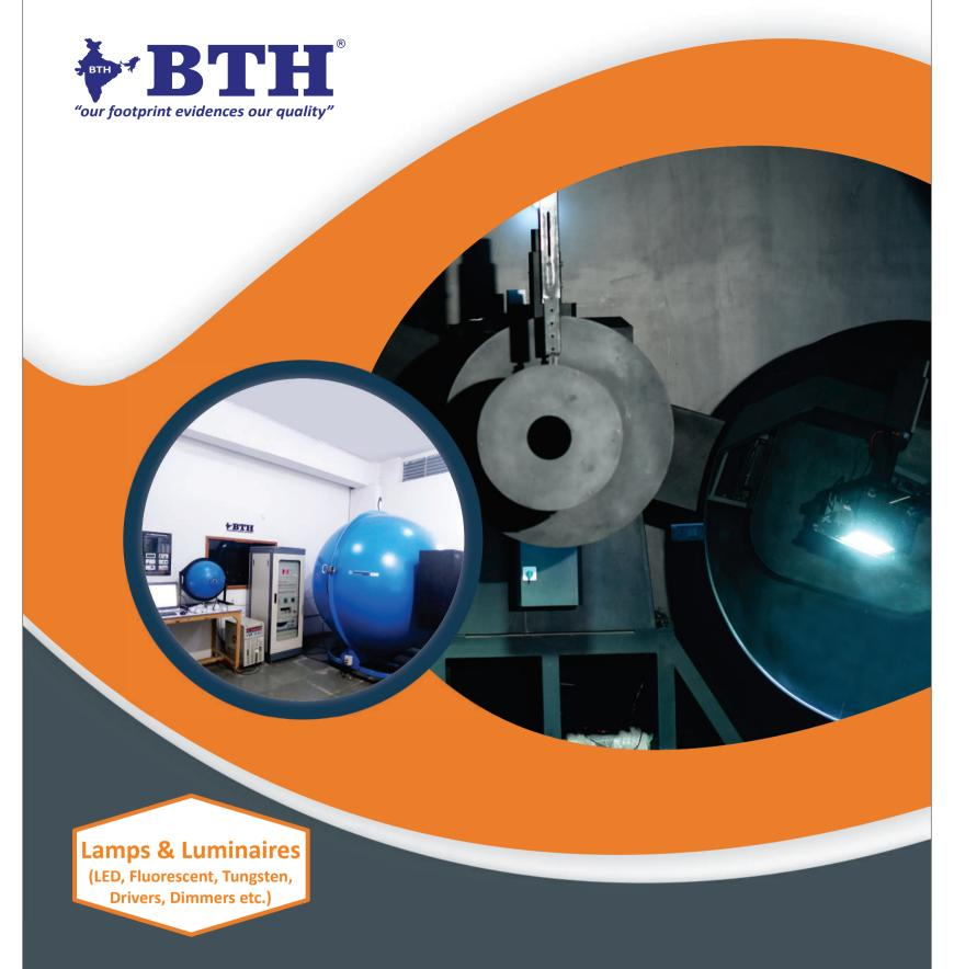
BTH has the state of art Photometry Laboratory with two sets of C-Type Goniophotometer.
